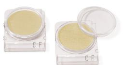
CompactDry<sup>™</sup> plates are suitable for detection and enumeration of microorganisms from foods and feeds, cosmetics and pharmaceutical samples, as well as for hygiene monitoring and contamination control in food-producing areas. Due to the chromogenic additives, colonies depict specific colouring, making them easy to interpret.
